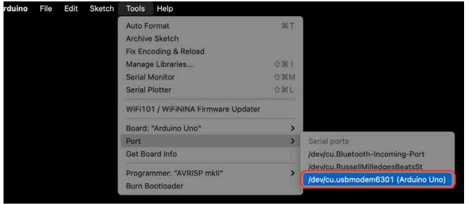
Enable the appropriate port for board in the Arduino IDE: Tools > Port >
