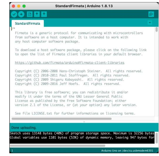
The Arduino Programmer informs you that it is "Done Uploading" the code to the Arduino board.
