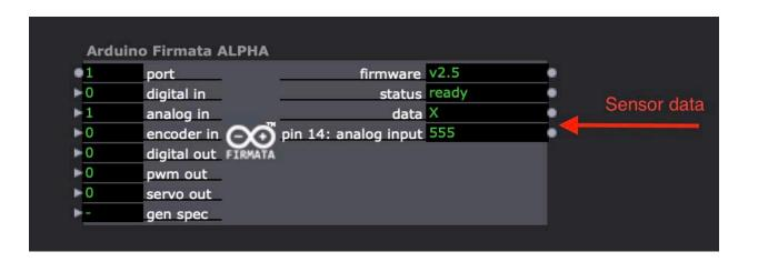
The sensor data is now routed to the Arduino Firmata module inside the Scene Editor of Isadora and can be linked into the patch.
