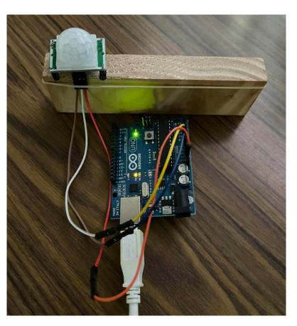
Go to the sensor and Arduino board and, with a jumper wire, set the Data and other pins of the sensor to the Arduino board pins specified by the Arduino Firmata module in Isadora.
