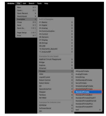
Select the Standard Firmata Example in the Arduino IDE: File > Examples > Firmata > Standard Firmata.
