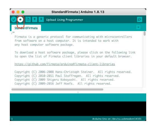
Upload the StandardFirmata code to the board using the Arduino IDE Programmer
