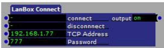
This is an adaption of jhoepffner's actor, I added the password as user input. After a connection is made, the LanBox command Common16BitMode is executed. For using this actor in a program make sure that the scene which contains the LanBox Connect actor is active. Otherwise you will loose the connection after a while. In my programs I include the LanBox Connect actor in the first scene, and in every subsequent scene I include an Activate Scene actor which points to this first scene.
