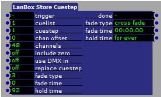
The use of this actor is to store DMX values into a cue step. The cue step will be created if not existing. The parameters of a new cue step are set by input values. The DMX values, which will be stored in the cue step are either the actual DMX output values or the actual DMX input values. So you can store what you see as a cue step or you can copy a step of another desk to a cue step of the LanBox.
