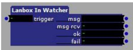
This actor is an adaption of the TCP In watcher. It listens to a TCP stream for only one input and only for one second. It is used in conjunction with a TCP send data actor, triggered at the same time. The LanBox In Watcher actor triggers „ok“, if it receives '>' or '\*' as first character of the returning string. It triggers „fail“ if it receives a '?' or after 1 second without an answer.
